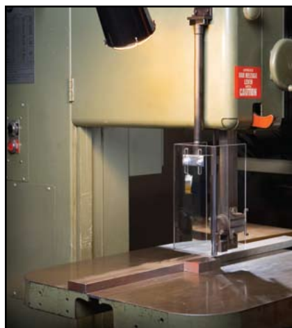
SHD-121510U shield assembly with an optional BKT-150 mounting bracket on a vertical band saw.
