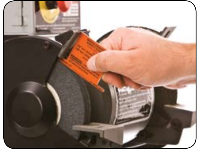
Checking a tongue that is not in compliance—the opening is greater than 1/4". (Shields removed for photo.)
