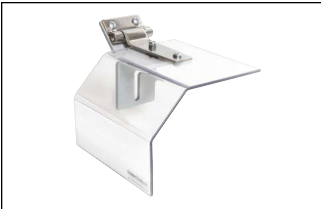
Part No. SHD-119L Assembly consisting of the 3/16"-thick polycarbonate shield, 1/4"-thick steel mounting bracket, hinge, fasteners, and safety sign.
