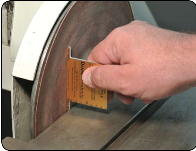
Checking a disc sander that is in compliance. (Shield removed for photo.)
