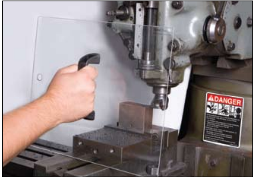
SHD-1512FP portable shield being used on a milling machine.
