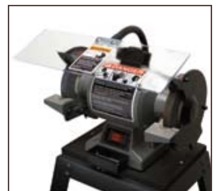
SHD-12165F shield assembly on a pedestal grinder.
