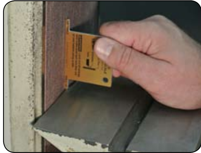
Checking a belt sander that is in compliance. (Shield removed for photo.)
