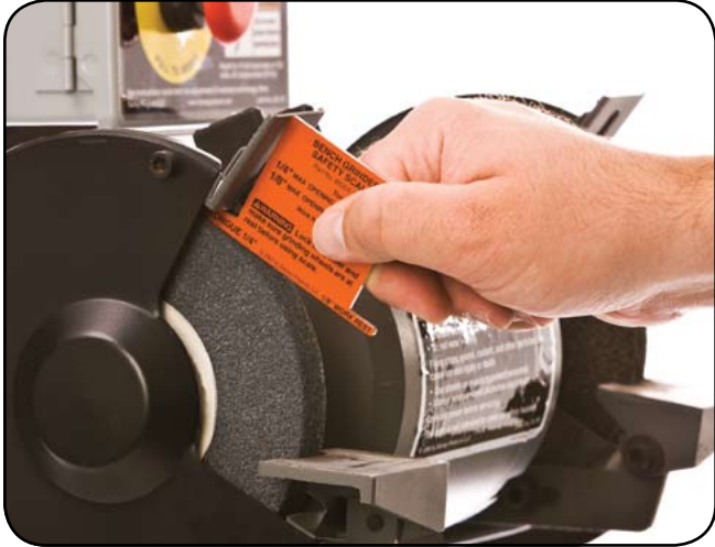
Checking a tongue that is not in compliance—the opening is greater than 1/4". (Shields removed for photo.)
