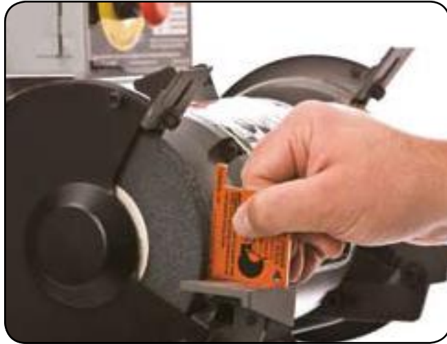
Checking a work rest that is not in compliance—the opening is greater than 1/8". (Shields removed for photo.)
