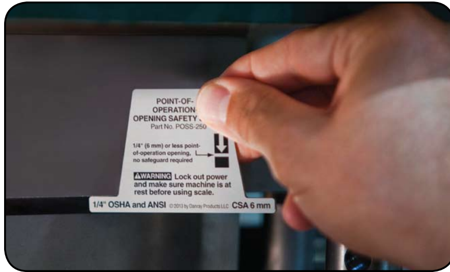
Checking a point-of-operation opening that is in compliance.
