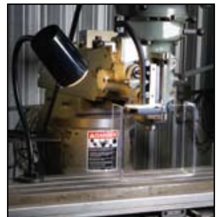
SHD-12169U shield assembly with an optional BKT-150 mounting bracket on a milling machine.
