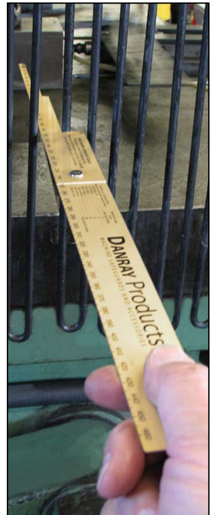
Checking a barrier guard that is in compliance.
